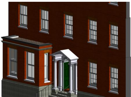
Correct building shape with major and minor details modelled – excludes ornate mouldings.
